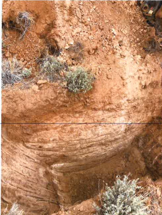
Test Pit #1 4-6" of top soil followed by silty clay loam to a depth of 8' with no rocks, no bedrock, no groundwater
