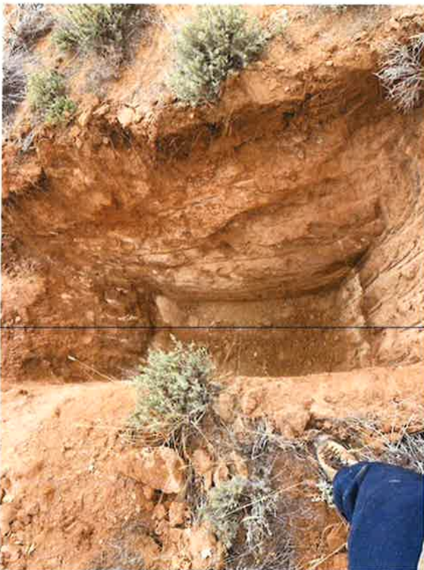
Test Pit #1 4-6" of top soil followed by silty clay loam to a depth of 8' with no rocks, no bedrock, no groundwater
