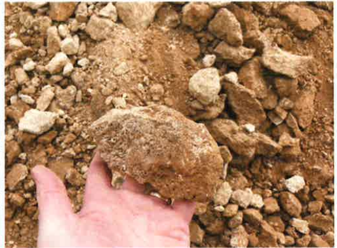
Soil maintained a blocky structure once excavated and the vertical blocky structure could be seen on trench side walls. Little to no rock.
