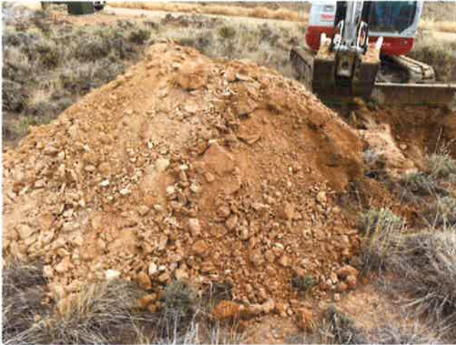
Soil maintained a blocky structure once excavated and the vertical blocky structure could be seen on trench side walls. Little to no rock.
