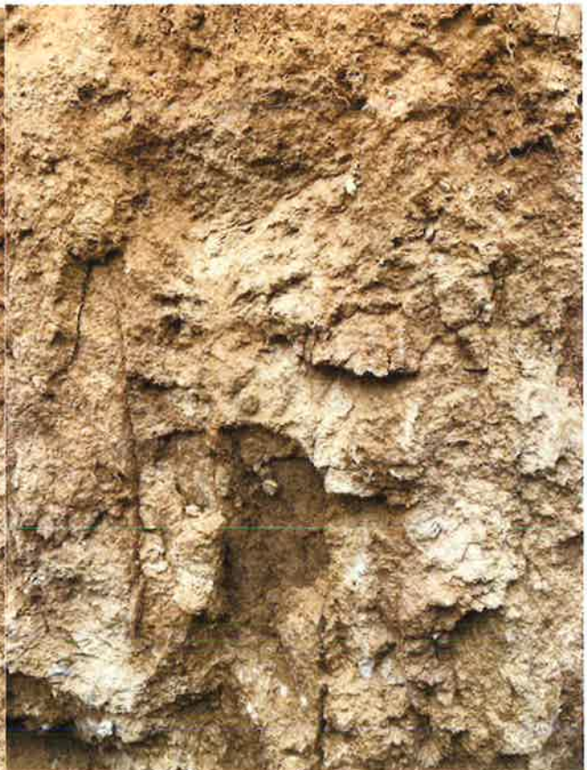
Soil maintained a blocky structure once excavated and the vertical blocky structure could be seen on trench side walls. Little to no rock.
