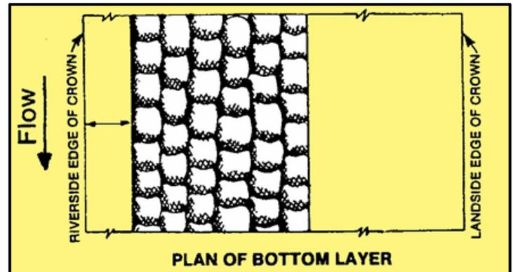
**Pyramid Placement Method** – The pyramid placement is used to increase the height of sandbag protection. Place the sandbags to form a pyramid by alternating header courses (bags placed crosswise) and stretcher courses (bags placed lengthwise). Stamp each bag in place, overlap sacks, maintain staggered joint placement, and tuck in any loose ends.
