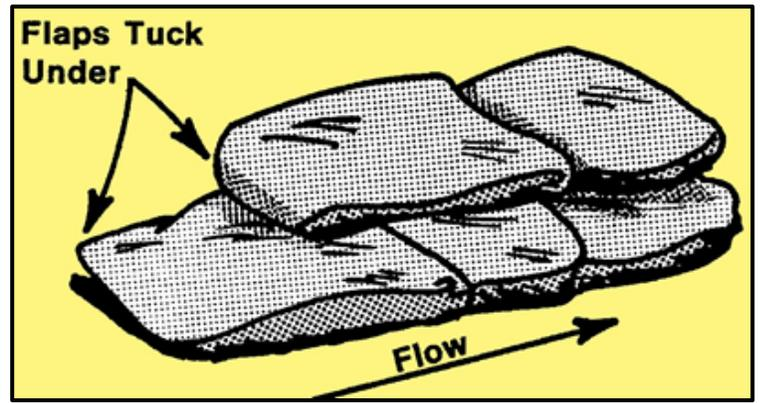
Stagger the joint connections when multiple layers are necessary. For unsupported layers over three (3) courses high, use the pyramid placement method (below).
